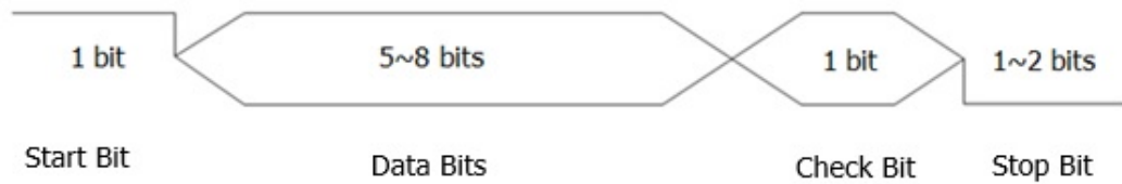
Figure 8.24 Schematic Diagram of RS232 Protocol
