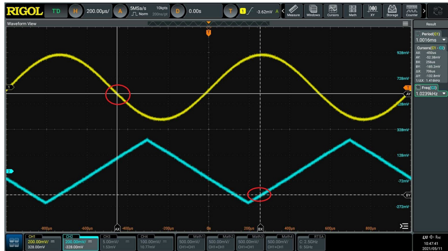
Figure 10.14 Track Measurement (after Horizontal Expansion)
